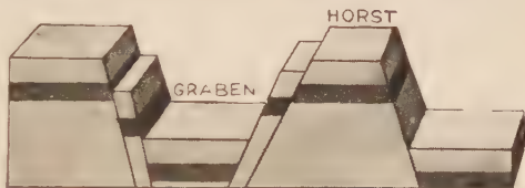
FIG. 257. — Block diagram showing the appearance and origin of a graben and horst.
